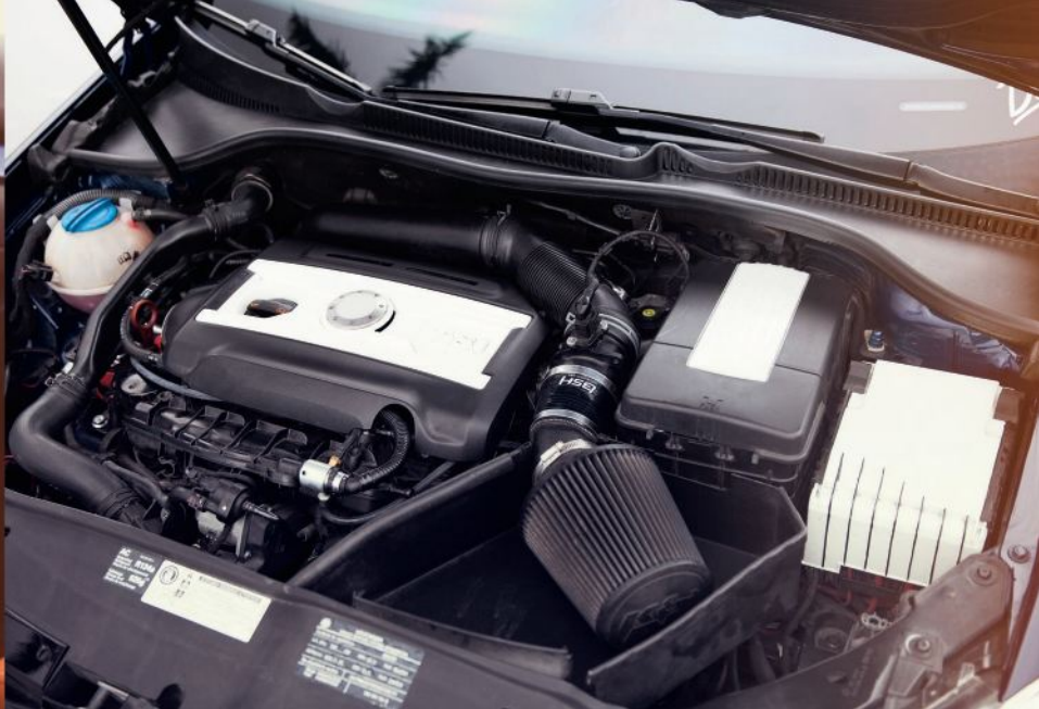
APR K04 big turbo, Forge Twintercooler, BSH intake and custom 3" exhaust are among the owner's favorite mods
