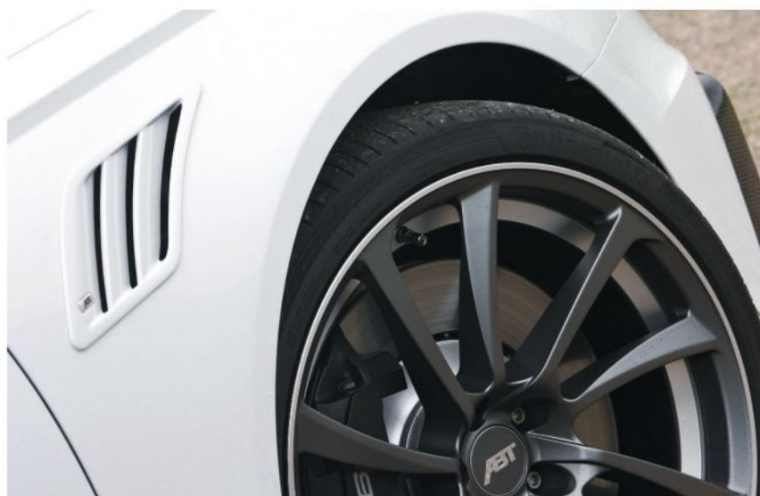
Chassis upgrades are restricted to 21" Abt wheels and Conti tires, with the tuner relying on the factory air suspension and carbon-ceramic brake rotors
