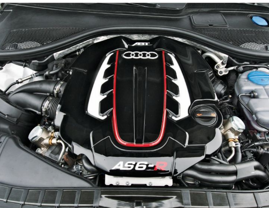
4.0L V8 biturbo makes 600hp and 553 lb-ft thanks to larger turbos and software tuning
