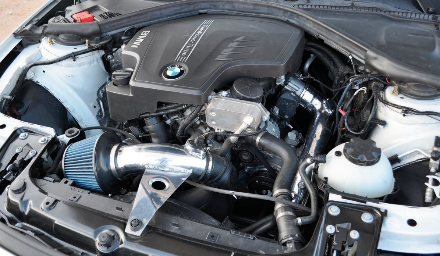
Evolution Racewerks intercooler, charge pipe, intake, downpipe, exhaust and Juicebox ECU produced 312whp and 355 lb-ft, making it the one of the most powerful 328i to date
