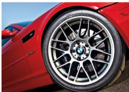
Six-piston Brembos were an early upgrade after the stock brakes melted on some high-speed runs
