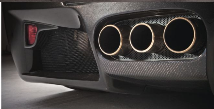
Custom titanium exhaust retains Ferrari's distinctive three-tailpipe design
