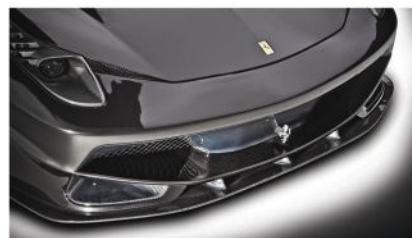
SVR front bumper is considerably deeper than stock part and constructed entirely from carbon fiber
