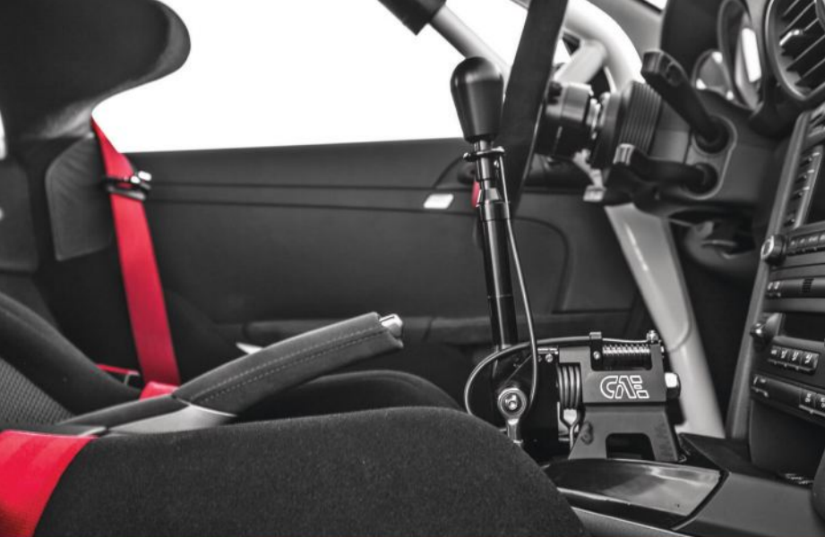
CAE shifter retains H-pattern but looks like sequential racing shifter
