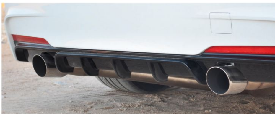
ER's dual exhaust sacrifices some low-end torque for high-RPM power. It sits in a 335i rear valance
