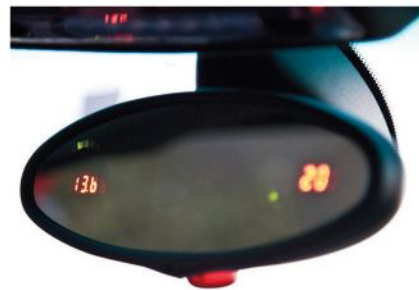
AEM wideband and boost gauge displays concealed in rearview mirror
