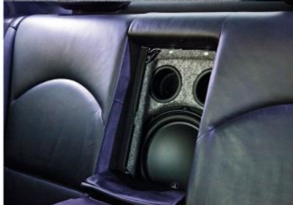
The car carries a significant sound system but it uses quick-release connectors for track-side removal
