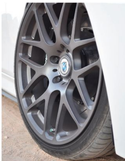
19" MORA wheels with Toyo tires, Brembo BBK and CKS coilovers
