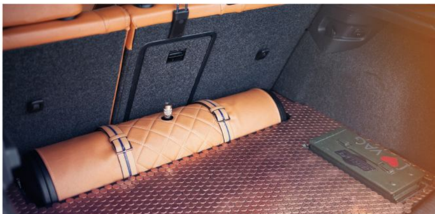
Eight-gallon air tank is submerged in the false floor that's covered in pennies
