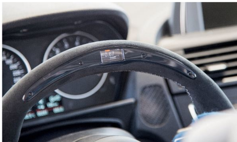
The majority of the driver information is selectable on the steering wheel display, which also provides shift lights
