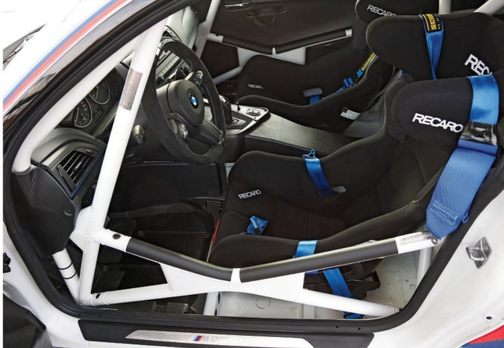
Full cage, Recaro seat, harnesses, M Performance steering wheel, carbon console and door cards are all that separate this interior from the production car
